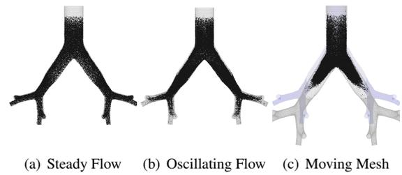
Figure 7: Particle ingress after 5s
