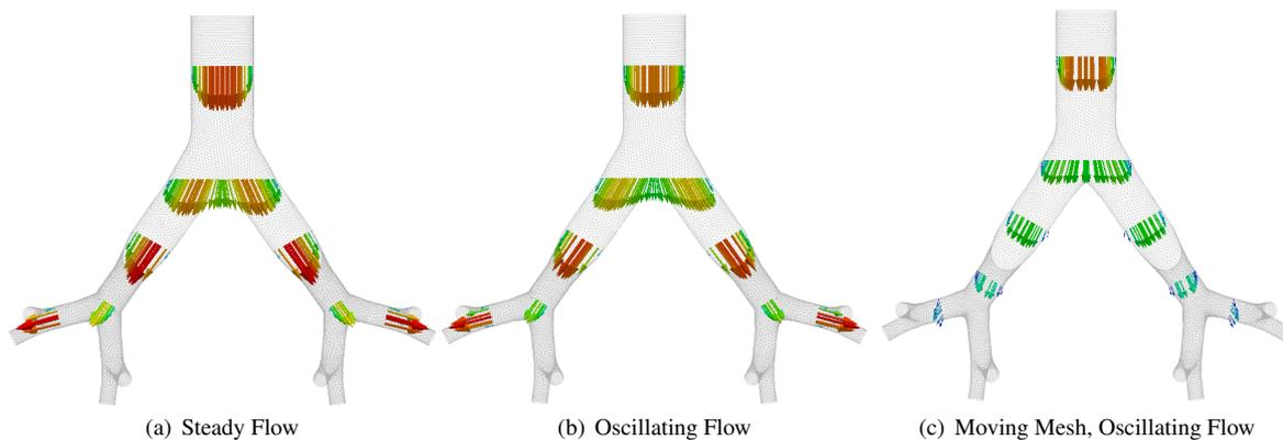
Figure 4: Velocity at various cross-sections at maximum inspiration.
